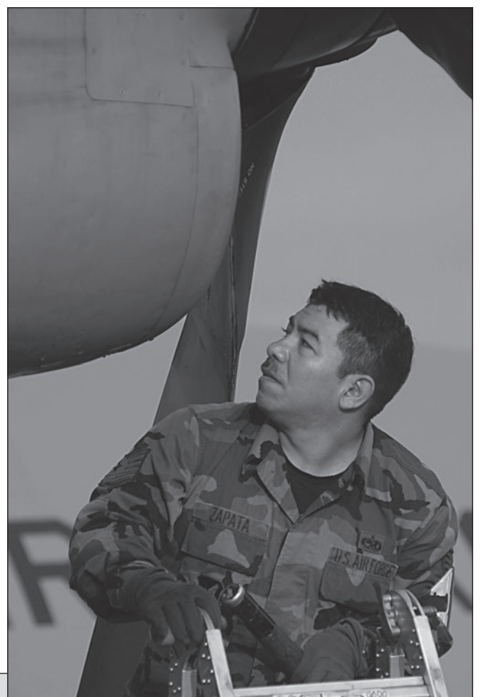
Tech. Sgt. Roberto Zapata, a C-130 crew chief with the 703rd Aircraft Maintenance Squadron, does inlet inspections before a flight. The inlet inspections are all included in the preflight inspections. An inlet inspection is an inspection of the engine for foreign objects that can damage the aircraft during flight.
