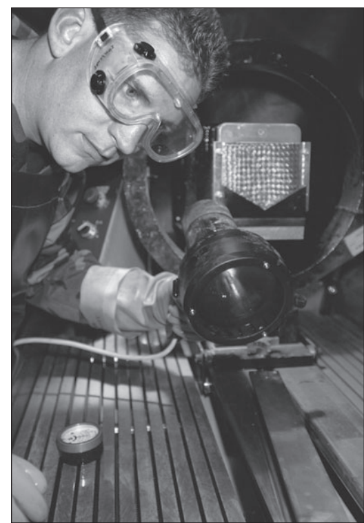
Tech. Sgt. Joseph Goff inspects an aircraft part for abnormalities. Sergeant Goff is the nondestructive inspection laboratory section chief at the 3rd Equipment Maintenance Squadron. The 3rd EMS is responsible for the long-term health of the C-130 fleet by completing a 13-day scheduled isochronal inspections at least once a year. The ISO maintainers look for structural cracks, broken and/or worn components and coordinate repairs. Aircraft are usually scheduled to deploy shortly after an ISO inspection to maximize its availability in the area of responsibility and prevent it from needing heavy, in-depth maintenance in theater, where the capabilities to do so are non-existent.
