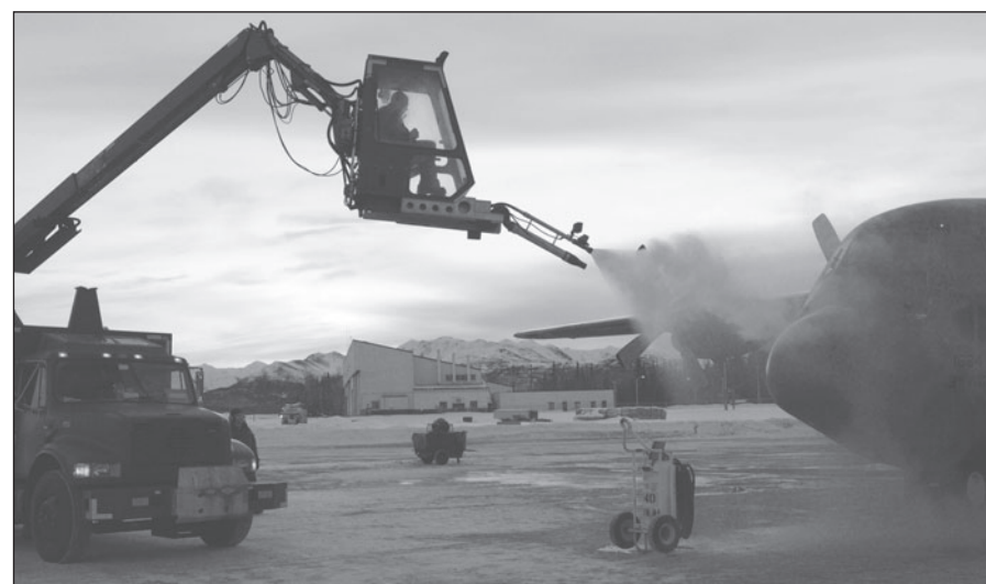
Senior Airman Steven Ferrin de-ices a C-130 Hercules before it takes off for a training exercise. Airman Ferrin is a crew chief for the 703rd Aircraft Maintenance Squadron, which maintains the 517 AS aircraft.
