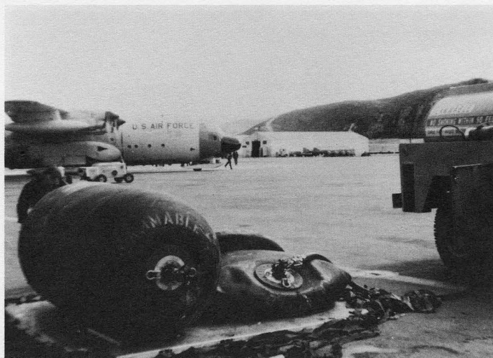
Before they switched to KC-97 fuel tanks, the Air Force used 500-gallon bladders to deliver diesel fuel to the sites. The bladders were strapped to pallets which were offloaded at the sites—a time-consuming job. (USAF Photo)
