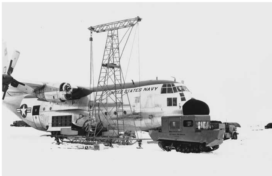
Left: The No.3 propeller was damaged during circular taxi tests at high speeds of approximately 30 to 50 knots. Nine days were required to transport a replacement prop from New Zealand to McMurdo because of high en route winds. When the new prop was installed, the engine was found to be damaged. The aircraft had to be flown to New Zealand for an engine change. (USAF Photo No. 61-2202) Left center: Cockpit view of C-130BL test aircraft showing installation of elevator force measurement control wheel in the pilot's position. (USAF Photo No. 61-2199) Left lower: Close-up front view of nose ski on the C-130BL. (USAF Photo No. 61-2195) Opposite: Three-quarter view of the C-130BL test aircraft at Williams Field, McMurdo Sound, Antarctica. (USAF Photo, Fitzwater Collection)
